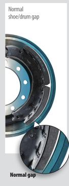
Heat from braking expands the drum & increases the gap
