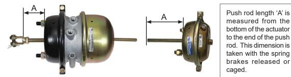
These heavy-duty push rods are manufactured from steel rods with an original diameter of 0.625 inches over the full length prior to threading. Standard push rods are manufactured from steel rods that are only 0.581 inches in diameter. As a result, the heavy-duty push rods are approximately 20% stronger than the standard push rod.
