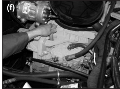
Inspecting the coolant hoses.
