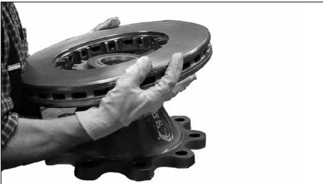
FIGURE 88 - INSTALLATION DU DISQUE DE FREIN
