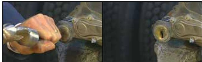
**FIGURE 63 - PERCER UN TROU DANS LE CAPUCHON DE LA TIGE DE GUIDAGE (12)**
