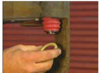
**FIGURE 83 - PLACER L'ANNEAU DE RETENUE DANS LA RAINURE DE LA TIGE DE GUIDAGE**
