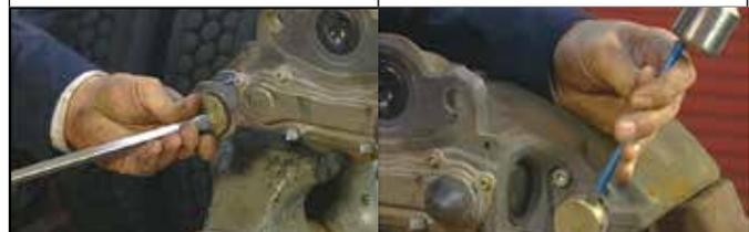
**FIGURE 65 - SOULEVER LE CAPUCHON DE LA TIGE DE GUIDAGE (12)**
