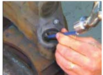
**FIGURE 73 - ENLEVER L'ONGLET QUI MAINTIENT LA DOUILLE EN PLACE**
