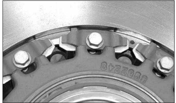
FIGURE 91 - ATTACHES INSTALLÉES
