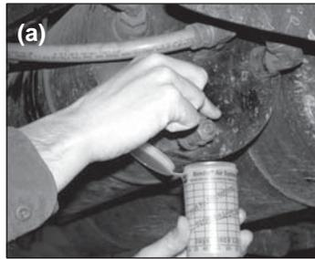
Drain all air tanks (reservoirs) into the Bendix® BASIC™ test cup. (Bendix kit P/N 5013711).
