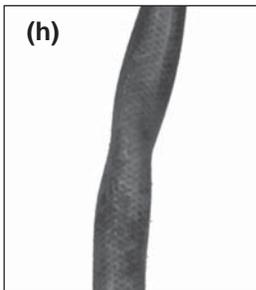
Partly collapsed inlet line shown.
