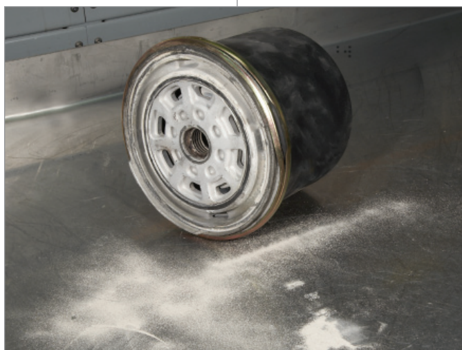
The desiccant of the knockoff cartridge turned to powder, contaminating the entire brake system.
