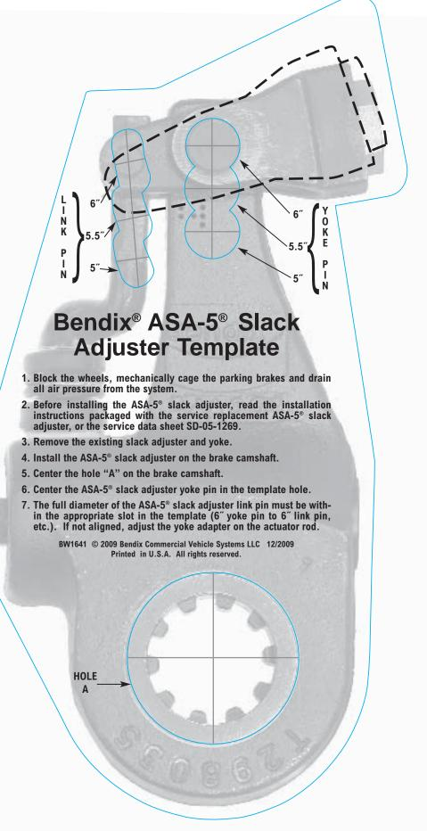
This template is not needed for the ASA-5® slack adjuster installation. Please refer to the installation instructions included with your product. This template can be used for assistance, if needed.
