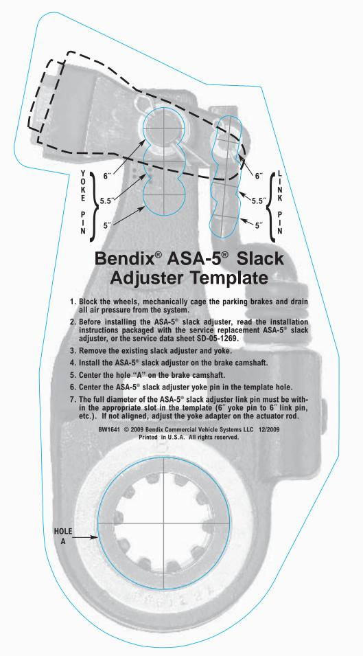
This template is not needed for the ASA-5® slack adjuster installation. Please refer to the installation instructions included with your product. This template can be used for assistance, if needed.
