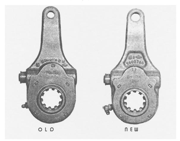
With the great emphasis being placed on vehicle weight reduction, Bendix has designed a new lightweight type 18 and 20 slack adjuster. The new unit, lighter than the current design, provides the same strength characteristics and is interchangeable with the older design unit.
