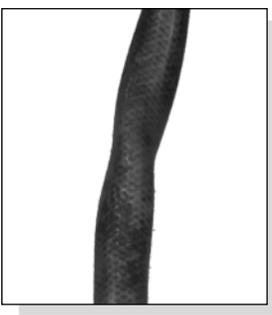
Partly collapsed inlet line shown.
