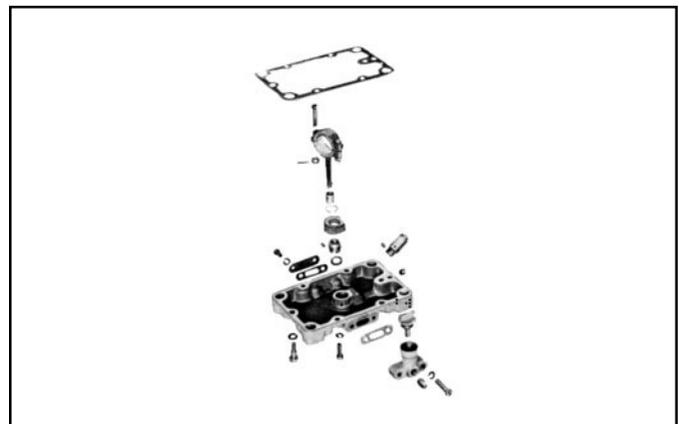
FIGURE 18 - BASE PLATE SELF-LUBRICATED TYPE COMPRESSOR
