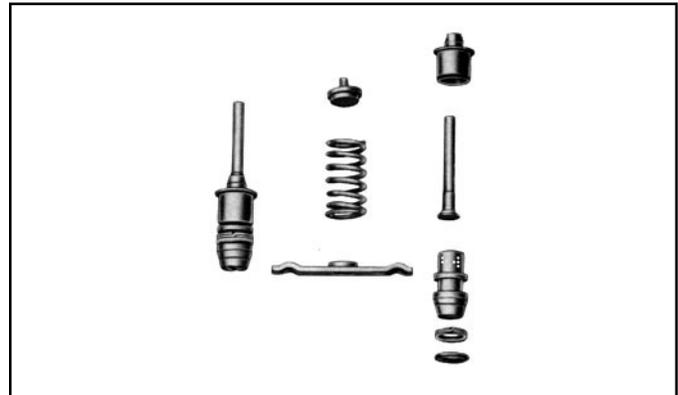
FIGURE 25 - UNLOADER MECHANISM
