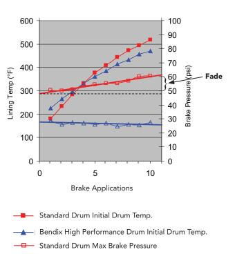
Bendix High Performance Drum Max Brake Pressure
