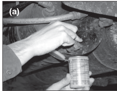
Drain all air tanks (reservoirs) into the Bendix® BASIC test cup. (Bendix kit P/N 5013711).
