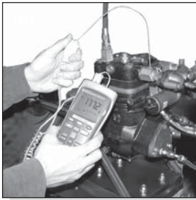
Testing the temperature at the discharge fitting.
