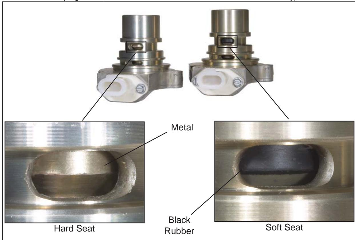
Figure 1 - Identification of Hard and Soft Seat Purge Valves
