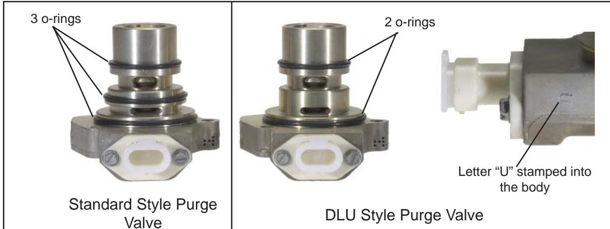
Figure 2 - Standard and DLU Purge Valves
