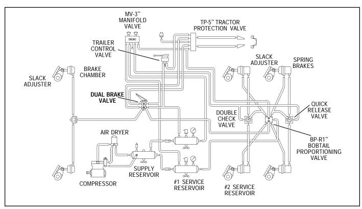
FIGURE 3 - TYPICAL PIPING SCHEMATIC
