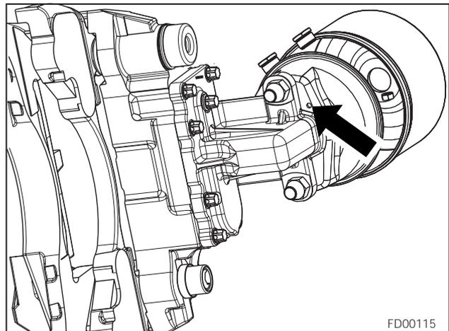
Attach the Actuator with new Nuts (self-locking EN ISO 7042) and torque tighten to 133<sup>+22</sup> ft.lbs. (180<sup>+30</sup> Nm).
