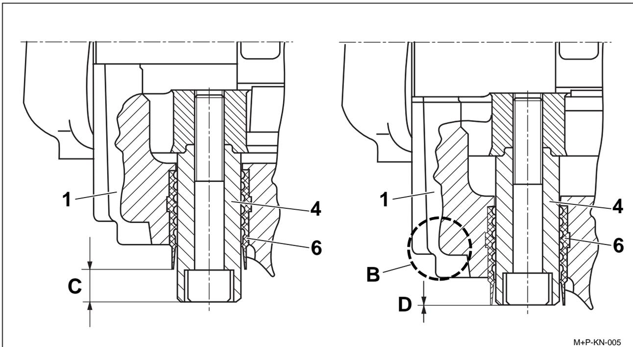
Pad conditions can be visually inspected without removing the road wheel by noting the position of the Floating Pin (4) in the Caliper (1).
