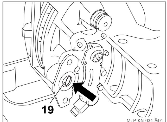
Attach Actuator with new Nuts (self-locking EN ISO 7042) and torque tighten to 133<sup>+22</sup> ft. lbs. (180<sup>+30</sup> Nm).
