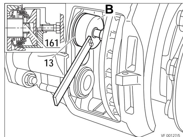
Using Tool B in reverse direction, the Tappet can be pressed on.
