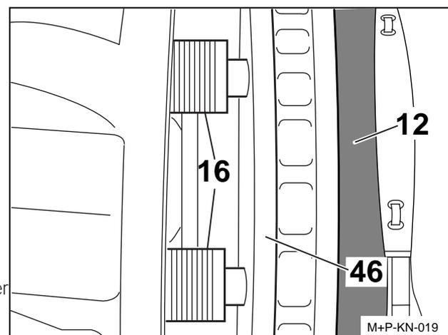
If Caliper is not installed on axle, put a spacer E (length = 2.76in. [70mm]) into the Caliper (1) to avoid overrunning of the Threaded Tubes (16) when adjusting them out (see illustration opposite). During adjusting, the threads can be checked for corrosion damage. In case of water ingress or corrosion, the Caliper must be replaced.
