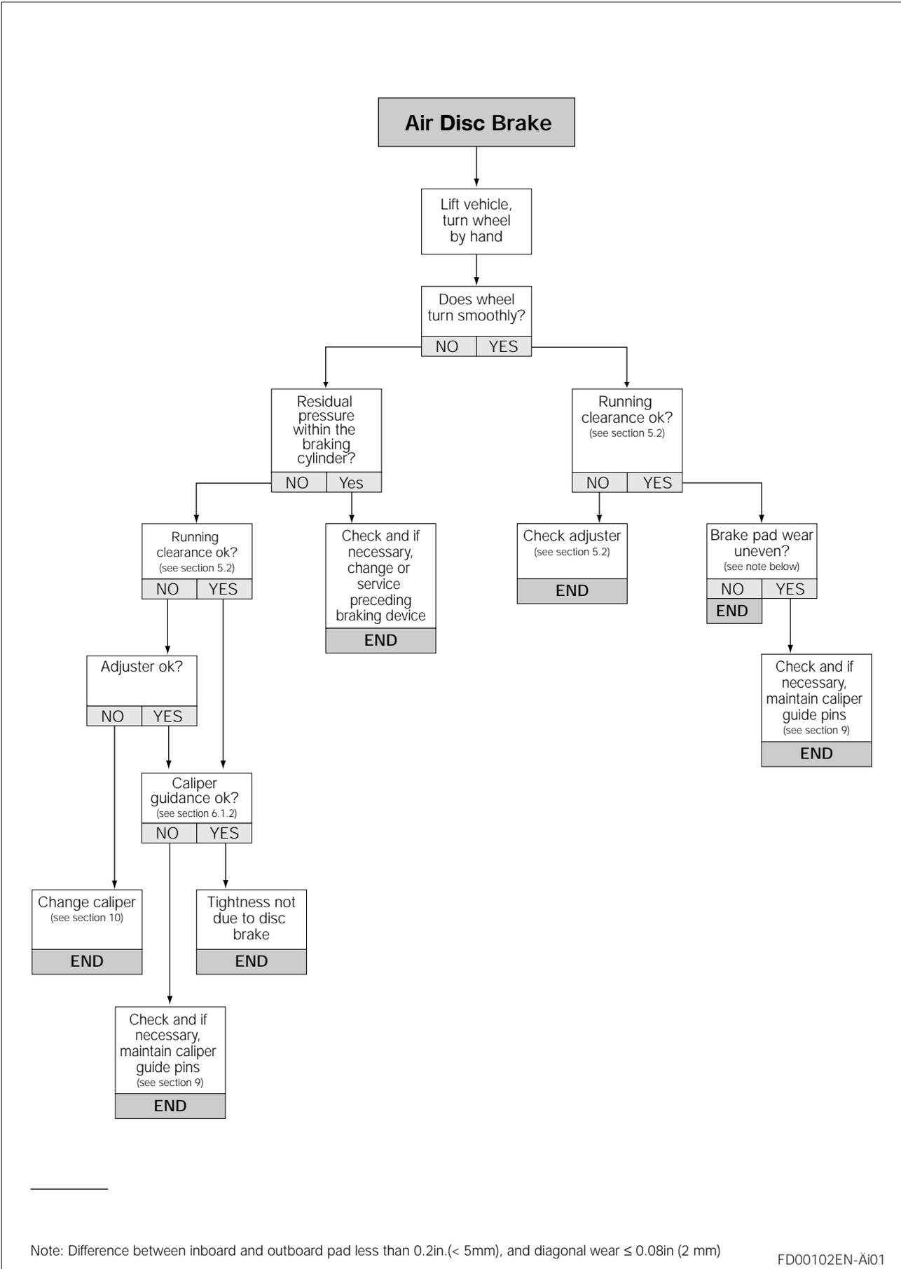
Note: Difference between inboard and outboard pad less than 0.2in.( $< 5\text{mm}$ ), and diagonal wear  $\leq 0.08\text{in}$  (2 mm)
