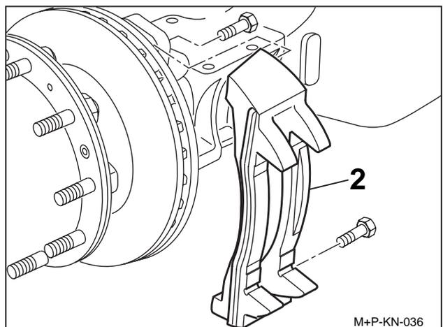
Attach the Caliper (see Section 10.2)
