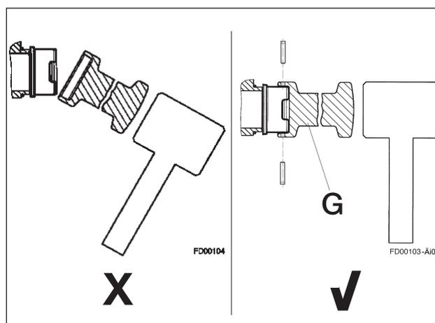
Assembly on the Caliper and Carrier removed from the axle:
