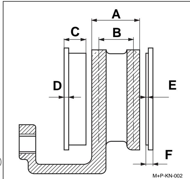
If wear dimension  $B \leq 1.53\text{in. (39 mm)}$  Rotor should be replaced together with Pads.
