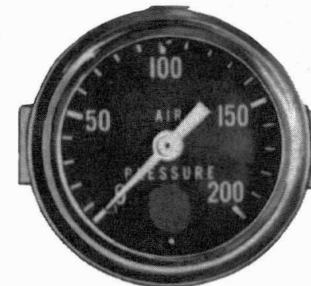
TYPE PG-1 PRESSURE GAUGE — DASH MOUNTED WITH ILLUMINATING SLOTS 2.28" Outside Diameter - Pressure Graduations 0 to 200 Lbs. Pc. No. 281265 COMPLIES WITH FMVSS #121 ONLY WHEN USED IN AIR BR. SYS. WITH COMPR. CUT-OUT PRESS. OF 115 P.S.I. OR MORE
